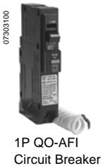
QO arc-fault circuit interrupters (AFCI) quickly detects a wide range of arc-fault conditions, recognizes the nature and specific wave-form of an arc fault and trips the circuit breaker. Traditional circuit breakers and fuses are designed to detect overloads and short circuits. Arc-fault circuit breakers are designed to detect overloads, short circuits and arc faults.
