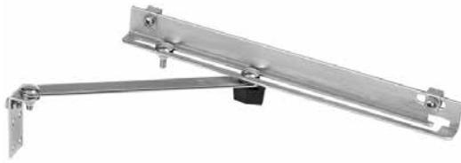
Door Stop Kit secures the door in the open position. Kit can be installed at the top or bottom of a door which opens horizontally. Door opening angle can be easily adjusted by means of a wing nut. Stop arm slides neatly out of the way when the door is closed. All parts are plated. Mounting hardware included.
