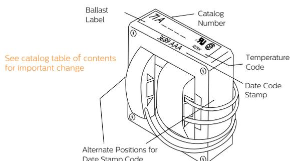
Philips Advance HID core & coil ballasts are date stamped on either the top surface or the side surface of the ballast core. The four-digit number represents the week and year of manufacture. The first two numbers indicate the week and the last two indicate the year the ballast was manufactured. The example shows a ballast manufactured during the 36th week of 1989. The three letters are a factory code.
